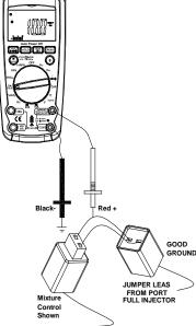
Connect black test probe to a good ground at the fuel injector or the negative (-) vehicle battery post.
